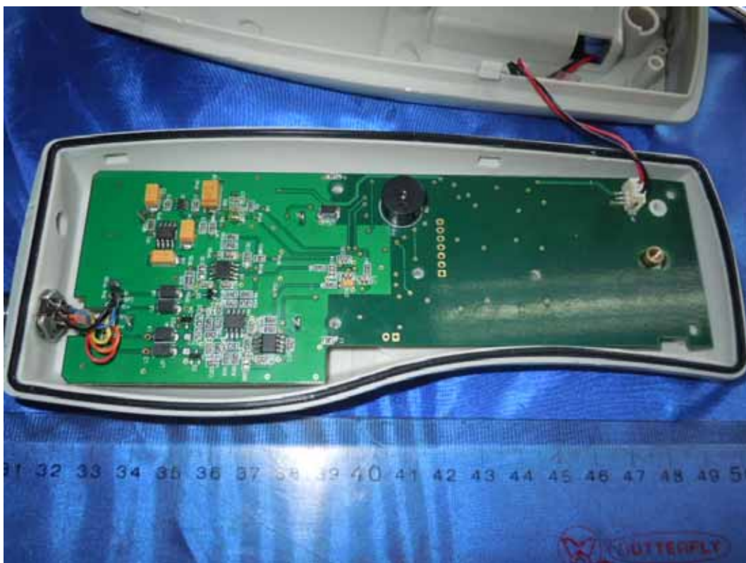
FIGURE 7 FIELD/LAB DISSOLVED OXYGEN AND TEMPERATURE INSTRUMENT (M/N: DO210) MAIN BOARD (SOLDERED SIDE)
