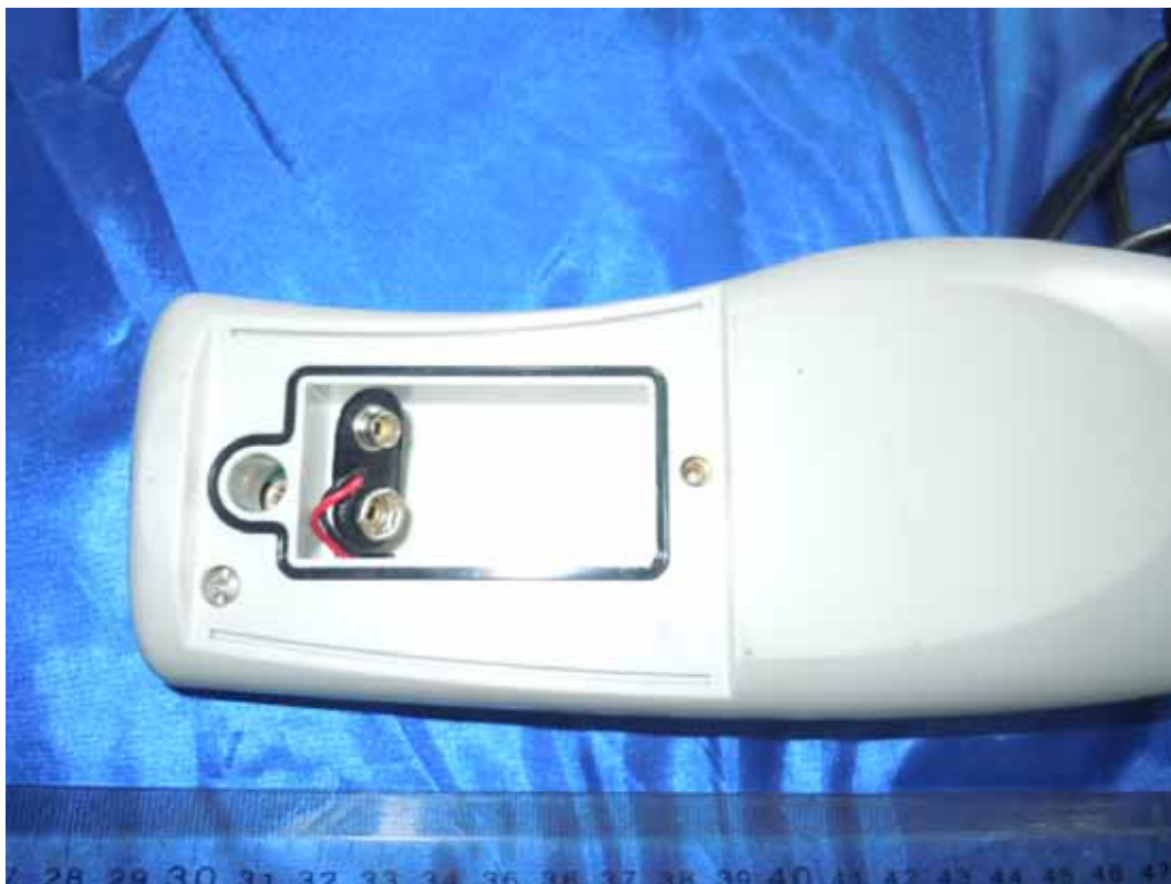
FIGURE 3 FIELD/LAB DISSOLVED OXYGEN AND TEMPERATURE INSTRUMENT (M/N: DO210) BATTERY POSITION
