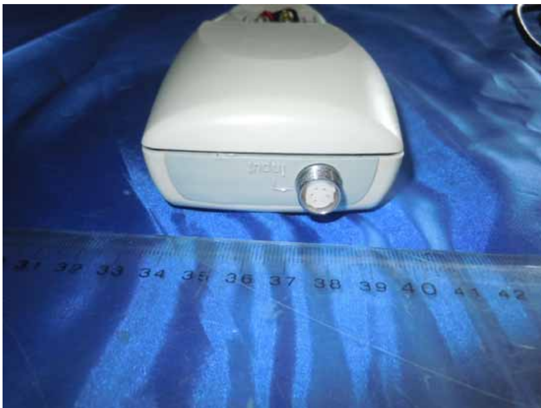
FIGURE 4 FIELD/LAB DISSOLVED OXYGEN AND TEMPERATURE INSTRUMENT (M/N: DO210) INPUT PORT
