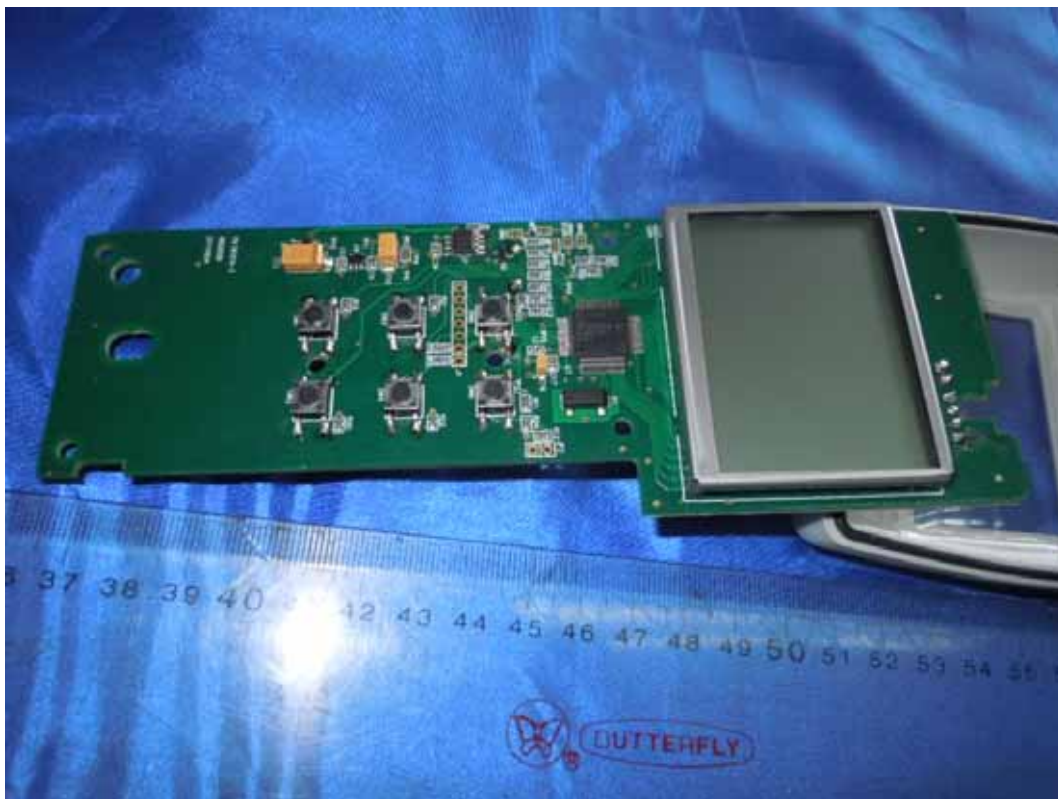
FIGURE 6 FIELD/LAB DISSOLVED OXYGEN AND TEMPERATURE INSTRUMENT (M/N: DO210) MAIN BOARD (COMPONENT SIDE)
