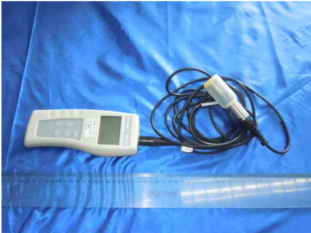
FIGURE 1 FIELD/LAB DISSOLVED OXYGEN AND TEMPERATURE INSTRUMENT (M/N: DO210) GENERAL APPEARANCE (FRONT VIEW)
