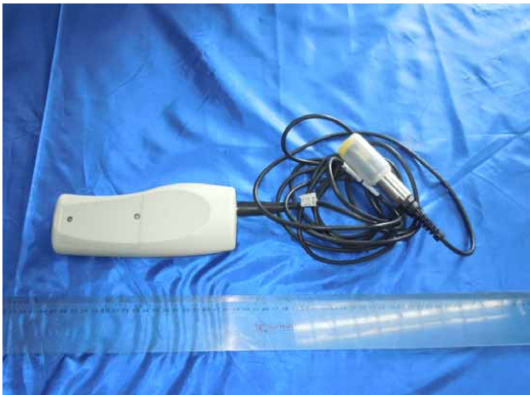
FIGURE 2 FIELD/LAB DISSOLVED OXYGEN AND TEMPERATURE INSTRUMENT (M/N: DO210) GENERAL APPEARANCE (BACK VIEW)
