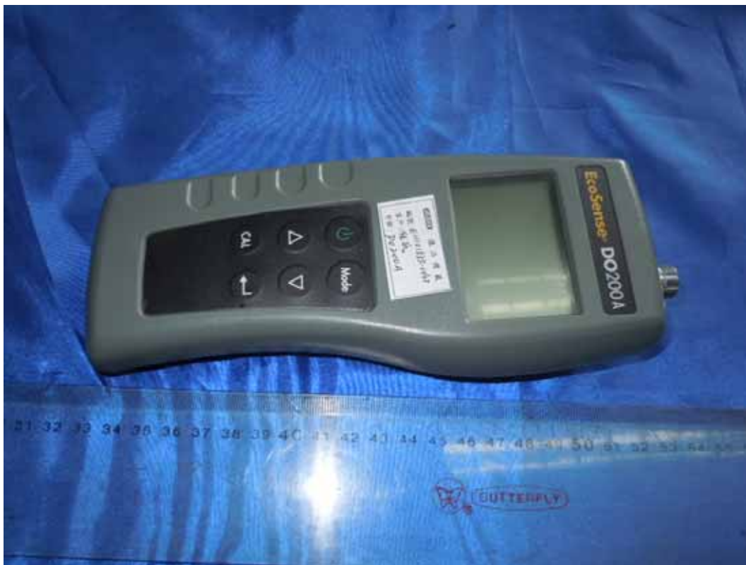
FIGURE 9 FIELD/LAB DISSOLVED OXYGEN AND TEMPERATURE INSTRUMENT (M/N: DO200A) GENERAL APPEARANCE (FRONT VIEW)
