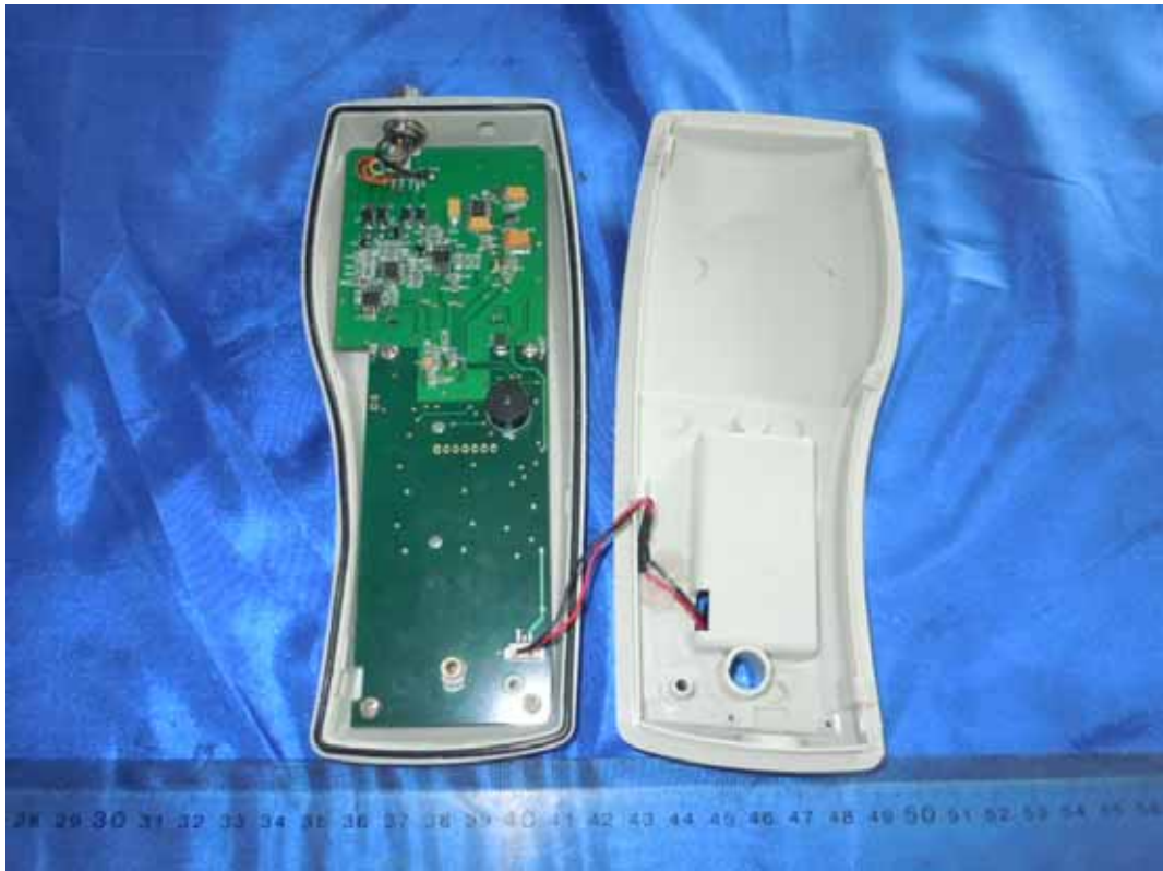
FIGURE 5 FIELD/LAB DISSOLVED OXYGEN AND TEMPERATURE INSTRUMENT (M/N: DO210) COVER REMOVED
